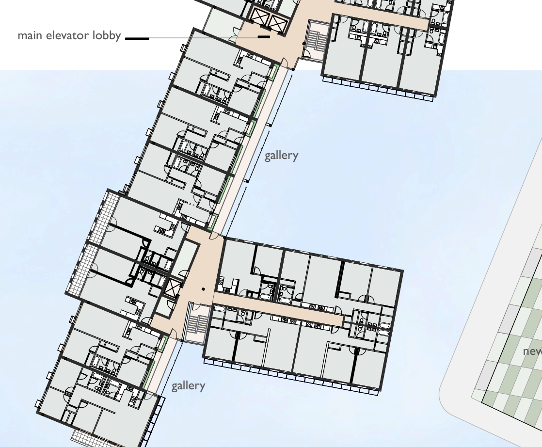
typical lower floor plan 1" = 40'-0"
